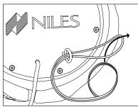
Figure 9 Security Cable Looping Through
